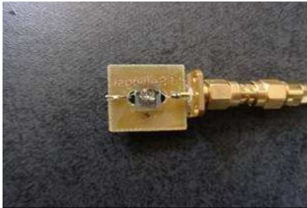
FIG. 3 – SAW sensor mounted on its connector.
