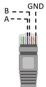
Figure 6: RS485 socket pinout
