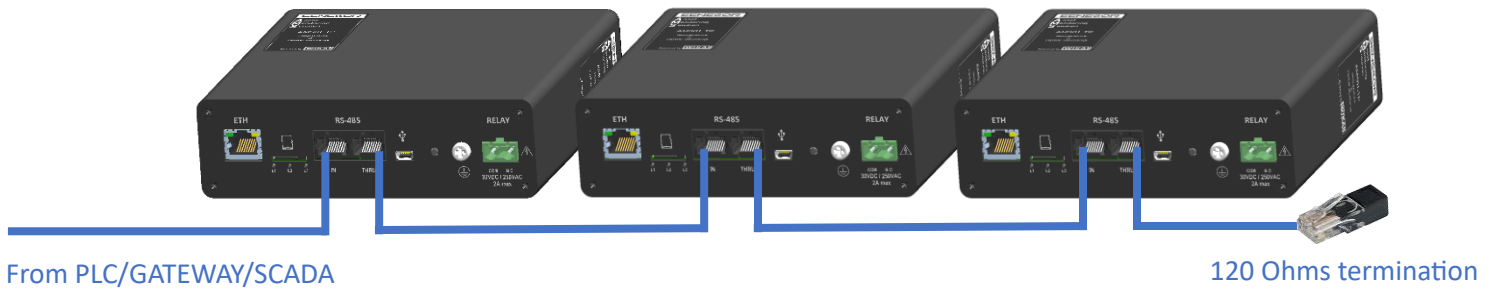
Figure 16: RS485 daisy chaining
