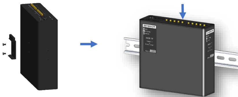
Figure 10: DIN rail fixation – Configuration 2
